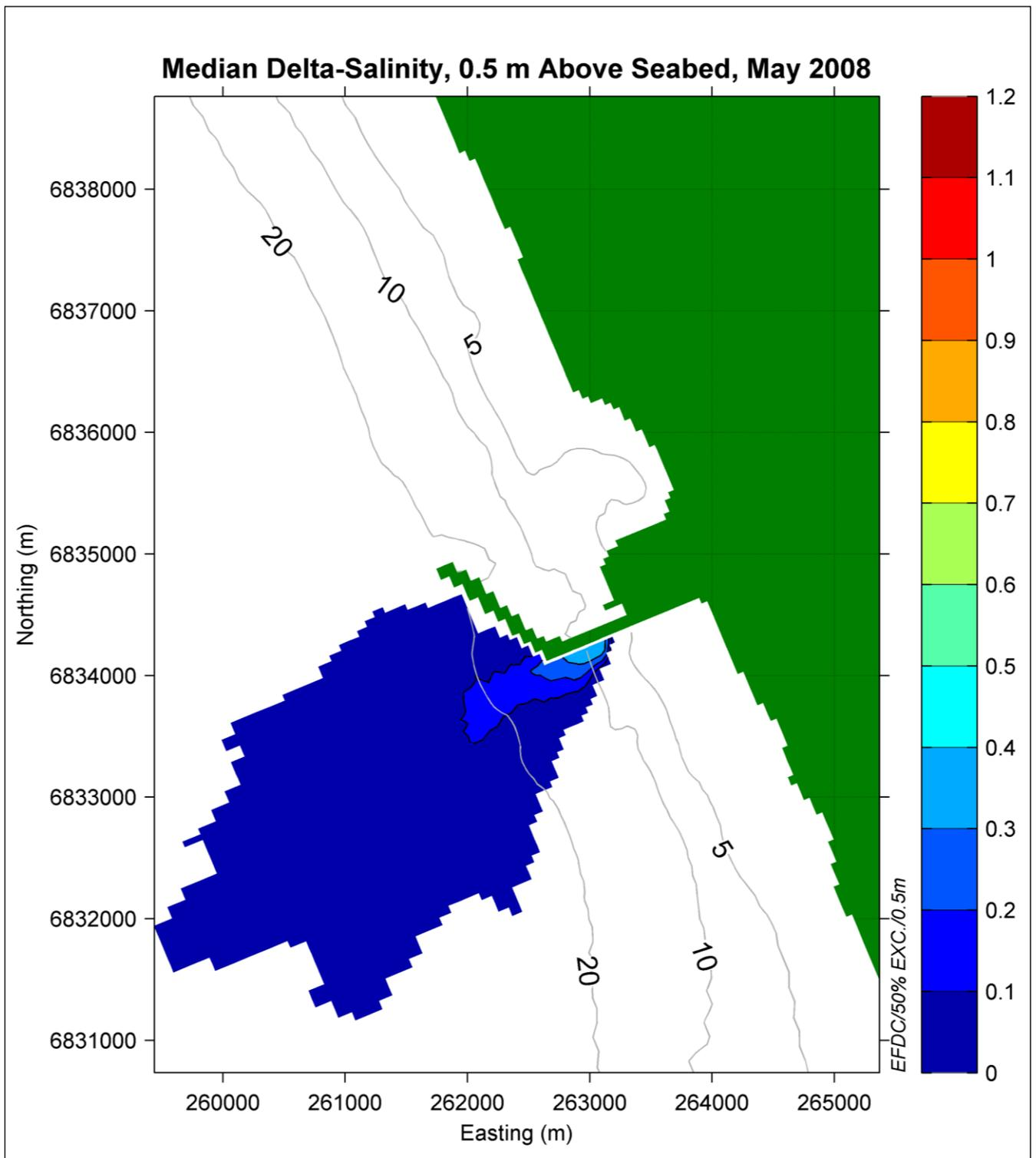
Figure 2 Spatial plot showing the predicted median salinity difference (proposed – existing) for the modelled May 2008 conditions. The coloured zones show the values indicated by the scale. Depth contours (5, 10 and 20 m) are also shown.
