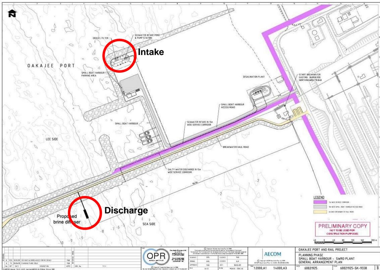
Figure 1 Location of desalination plant intake and discharge sites applied in the model.
